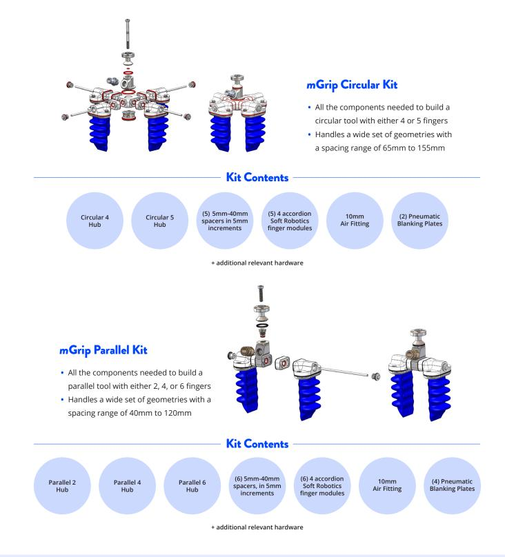
*m*Grip kits are offered in both a Standard (Aluminum) and Food Safe (Stainless Steel) option. Food Safe mGrip kits are compliant with (EC) 1935:2004 and meet the requirements of the United States FDA Codes of Federal Regulation 21 CFR concerning materials intended for repeated food contact.
